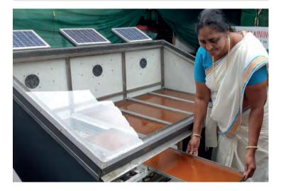
**Climate impact:** Using solar energy has a direct mitigation benefit and reduces dependence on fossil or bio fuels. With one solar dryer, about 1 t. of liquid and 2.6 t. of semi-liquid raw materials can be dehydrated annually to produce mango bars, fruit candy, etc. This saves 1.2 t. of firewood per year. Additionally, it reduces rotting of fresh fruits, minimizing methane emissions by approximately 20 kg/ton. About 5-6 t. of material can be composted, sequestering 1 t. CO2 more.
